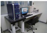
Desktop Scanning Electron Microscope (charge up reduction)
