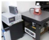
Shaker (max. acceleration: 20G)
